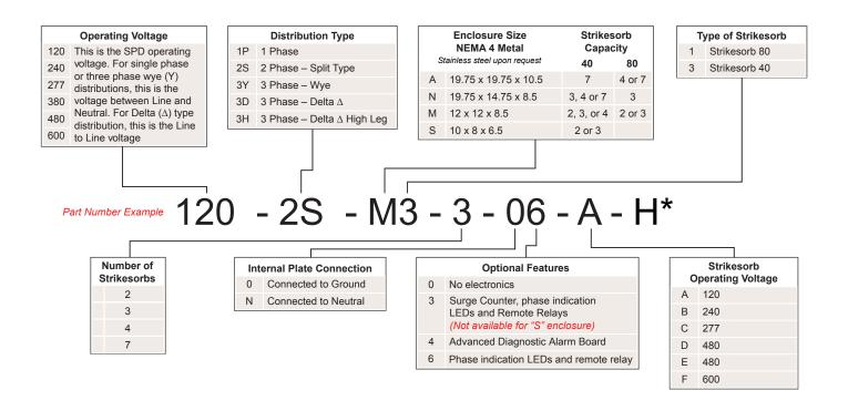
\*For a stainless steel enclosure specify "-SS" in place of the "-H" indication which is for the standard painted NEMA 4 enclosure.
